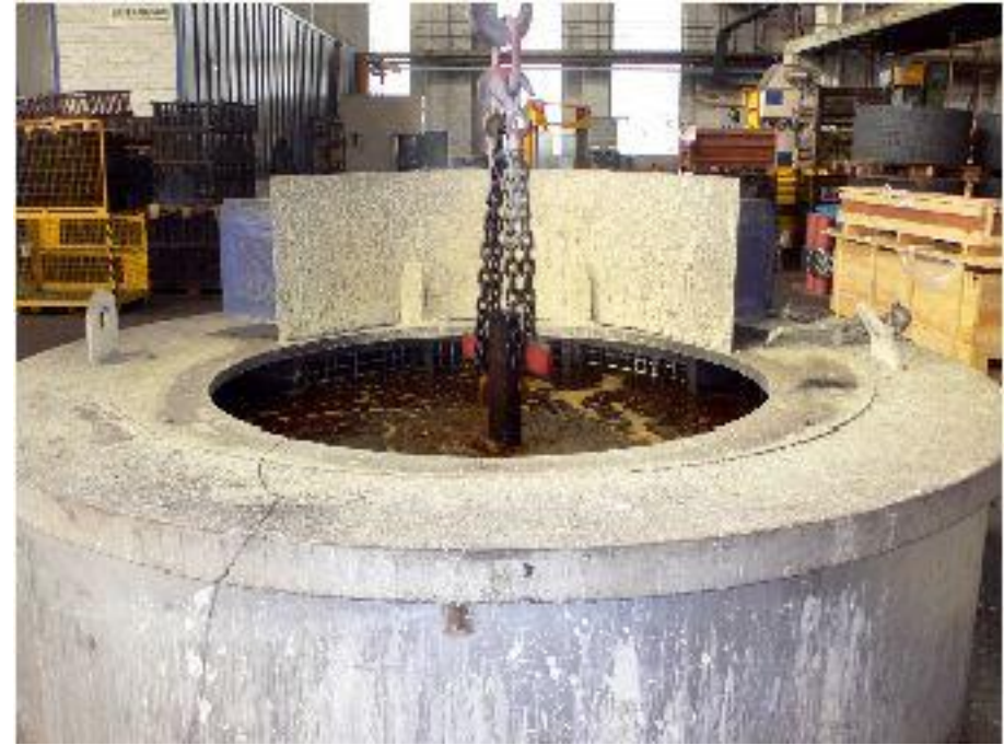
Fig. 2 : Bath II low-temperature salt-bath for isothermal treatment.
