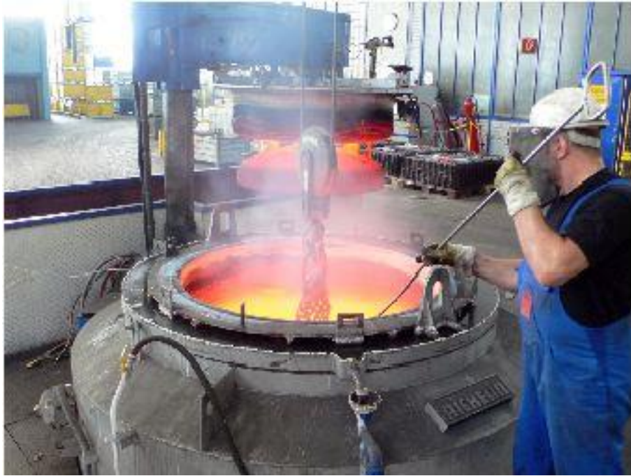
Fig. 1 : Salt bath I -austenitisation heat treatment.
